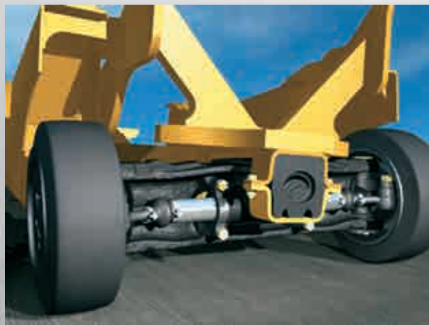
Above: HSM™ (Hyster Stability Mechanism) reduces truck lean in turns, improving lateral stability. The design allows for superior travel over uneven surfaces.
