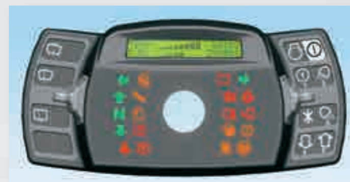
Above: The advanced integrated dash display uses a non-reflective, backlit LCD screen and 21 indicator lights provide information at a glance in all lighting conditions.
