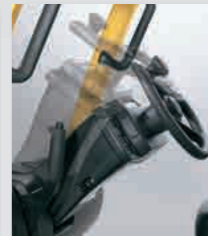
Left: The standard 30cm diameter steering wheel with spinner knob features an infinitely adjustable tilt steering column. Below: The rear grab handle provides an excellent hand hold for reverse driving while giving easy access to the auxiliary horn button.
