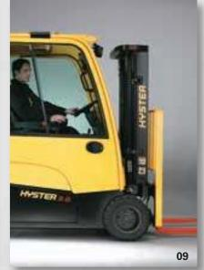
07 1.5 & 1.6T models are available with a Vista Plus mast, with 300mm between mast channels.
